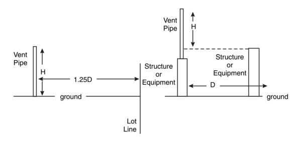
H = Minimum height in feet (mm) of vent pipe above the ground or above any structure or equipment within distance (D) where personnel might be present.
